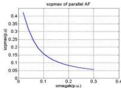
Fig. 9. Required compensating power depending on the frequency of voltage fluctuations for APF [3]
