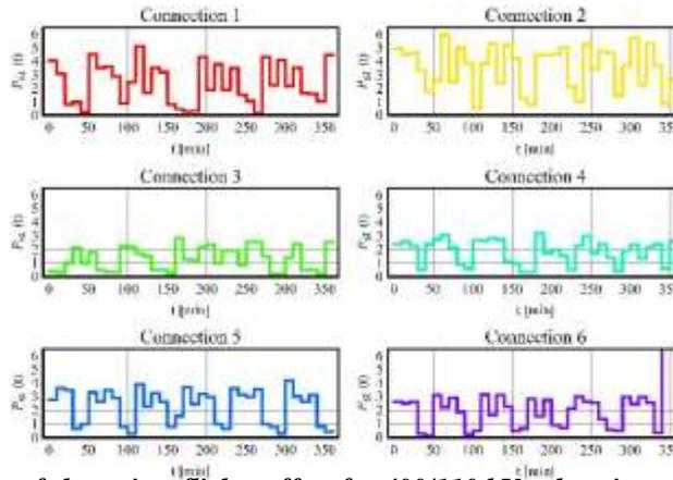
Fig. 4. Measurement of short-time flicker effect for 400/110 kV substation suplyment.
